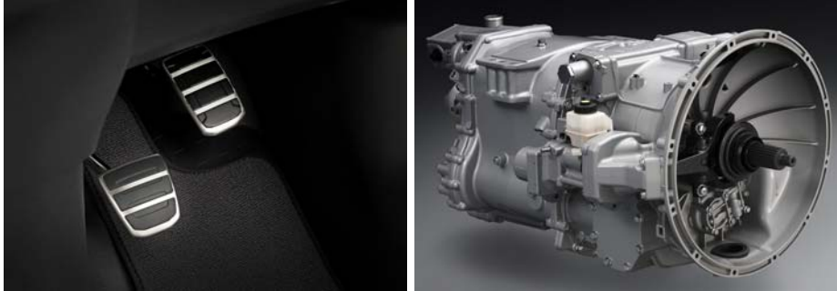
Fully automated Scania Opticruise with electro-hydraulic clutch control
